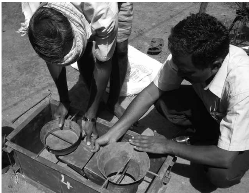
INNOVATE A smokeless chulha (traditional stove) is assembled in the village of Nayakanahatti. Naveen Lakshmipathy, the S 3 IDF team, and their partners constantly sought to explore innovative solutions.
